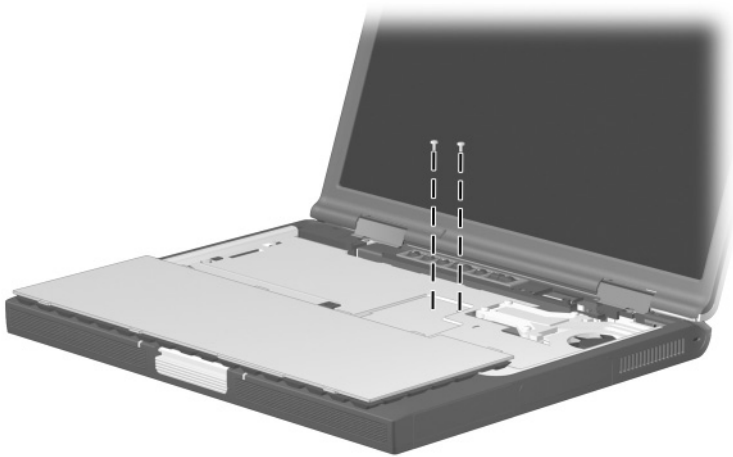
Figure C-7. Phillips M2.0 × 4.0 Screw Locations
